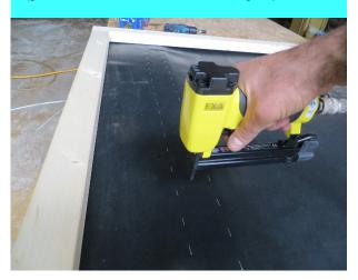
6. Turn the frame over and tighten the rubber (about 30-50 mm) and fix provisionally at the corners
