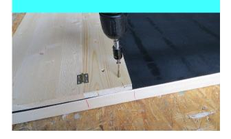
5. Turn the frame upside down and secure the rubber to the board over the door so that no wrinkles are left (you don't have to stretch yet)
