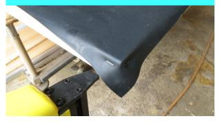
7. Now tighten the rubber and secure it provisionally to the side.
